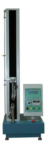
This machine is used to test tension, compression, bend, shearing force, adhesion, peeling force, tear strength, etc. of specimen, semi-product and finished product in the field of rubber, plastic, metal, nylon, fabric, paper, aviation, packing, architecture, electric appliance, automobile, etc., which are the basic facilities for input quality control, physical inspection, material research.
